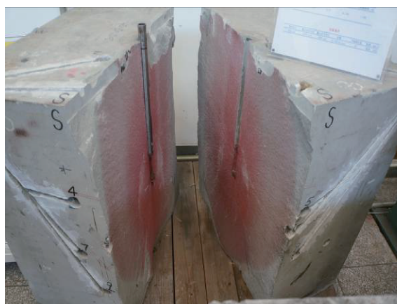
图1 裂缝不发育的岩心水力压裂后以单一裂缝为主 Fig. 1 A picture showing the dominant single fractures under hydraulic fracturing in the core featuring less developed fractures
