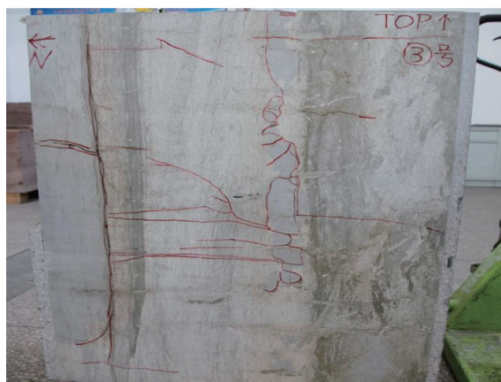
图2 微裂缝发育的岩心水力压裂后可见复杂的裂缝系统 Fig. 2 A picture showing a complex fracture network under hydraulic fracturing in the core featuring well developed micro-fractures
